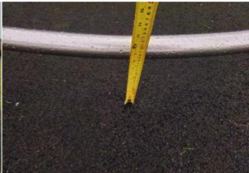
Finding: The height to the underside of the rim is less than Action: Monitor - No remedial work recommended 400mm and fails the requirements of BS EN 1176 Part 5
