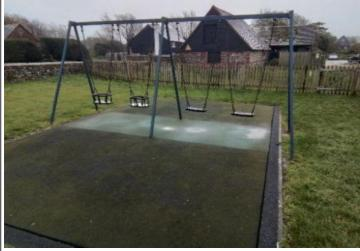
**Finding:** The surfacing width under the seat/s is / are less than 875mm when measured from the centre of the seat outwards, and fails the requirements of BS EN 1176 Part 2
